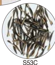
Material: S53C V=500m/min. f=0.25mm/tooth S=10000min -1 F=10000mm/min.
